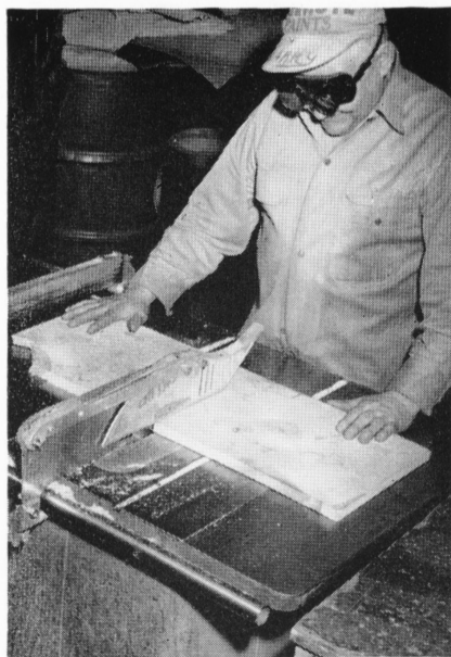
Harry Skrapolsky, of North Mill Finishing, uses a circular saw which is properly guarded. Notice the safety glasses and position of his hands.
